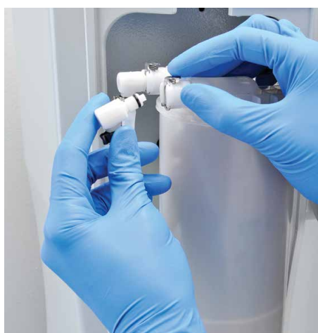
Rapid cartridge change with Aquastop quick-connect design
