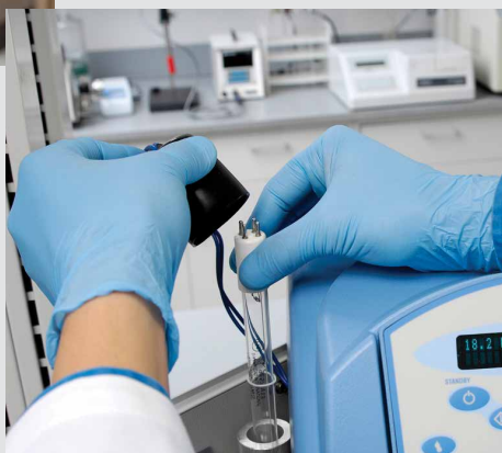
Changing the UV lamp protects the system against microorganisms and oxidizes organic compounds in the feed water, allowing for TOC levels of less than 5ppb
