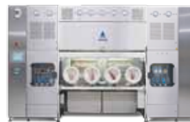
4 glove Isolator with 2 air locks
